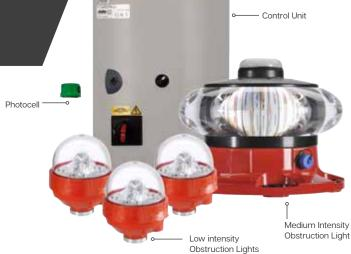
The Avlite ICAO I-2 Obstruction Lighting kit is a full turnkey solution for I-2 structures between 45 and 106 metres above ground. The kit consists of 1 x Red Medium Intensity Obstruction Light, 3 x Low Intensity (LI) Obstruction Lights, all necessary junction boxes and a central control unit. The I-2 Obstruction Kit is available in universal AC or DC input power configurations.
