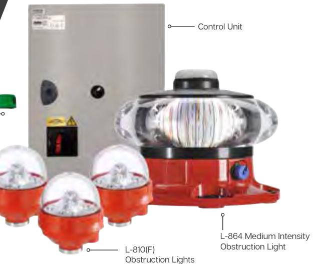
The Avlite FAA A-1 Obstruction Lighting kit is a full turnkey solution for A-1 defined structures between 150 and 350 feet. Consisting of 1 x L-864 Red Medium Intensity Flashing Beacon, 3 x L-810(F) Obstruction Lights, all necessary junction boxes and a central control unit. The A-1 obstruction kit is available in universal AC and DC input power configurations.
